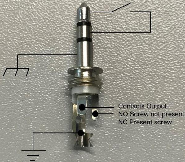
Possibility to connect the chassis frame directly to the ground
